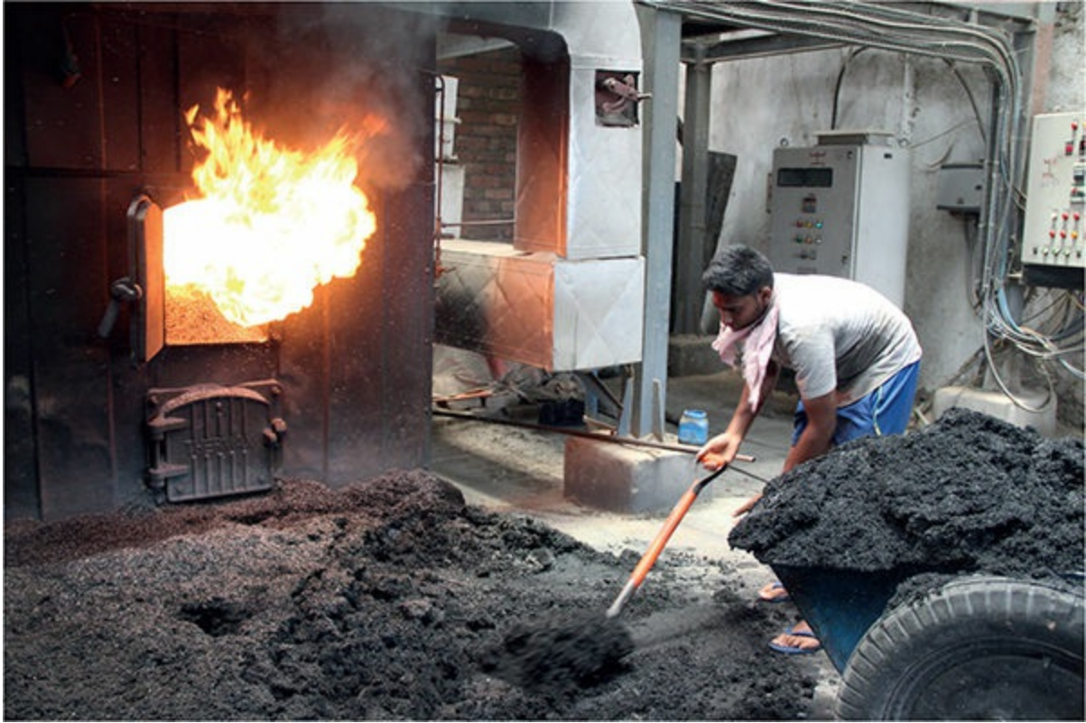
Workers in the process of helping Prabhu convert wheat chaff into sustainable energy at the Singur factory.
